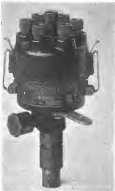
Latest type of Remy ignition unit and diagram of the breaker. The arm A is a light steel stamping
